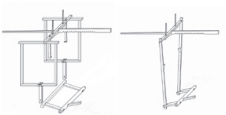
滑框和连杆的动力传动示意图 Power transmission diagram of sliding frames and connecting rods
