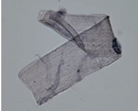
第一层背纸竹纸显微形貌 The microscopic morphology of the first layer of backing paper (Bamboo fiber)
